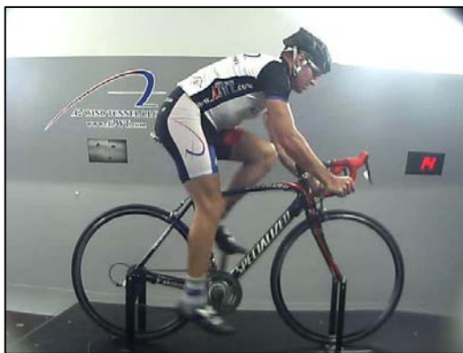
0 deg yaw aerodynamic test of road configuration at the A2 Wind Tunnel
