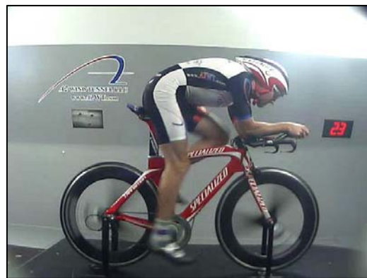
0 deg yaw aerodynamic test of time trial configuration at the A2 Wind Tunnel
